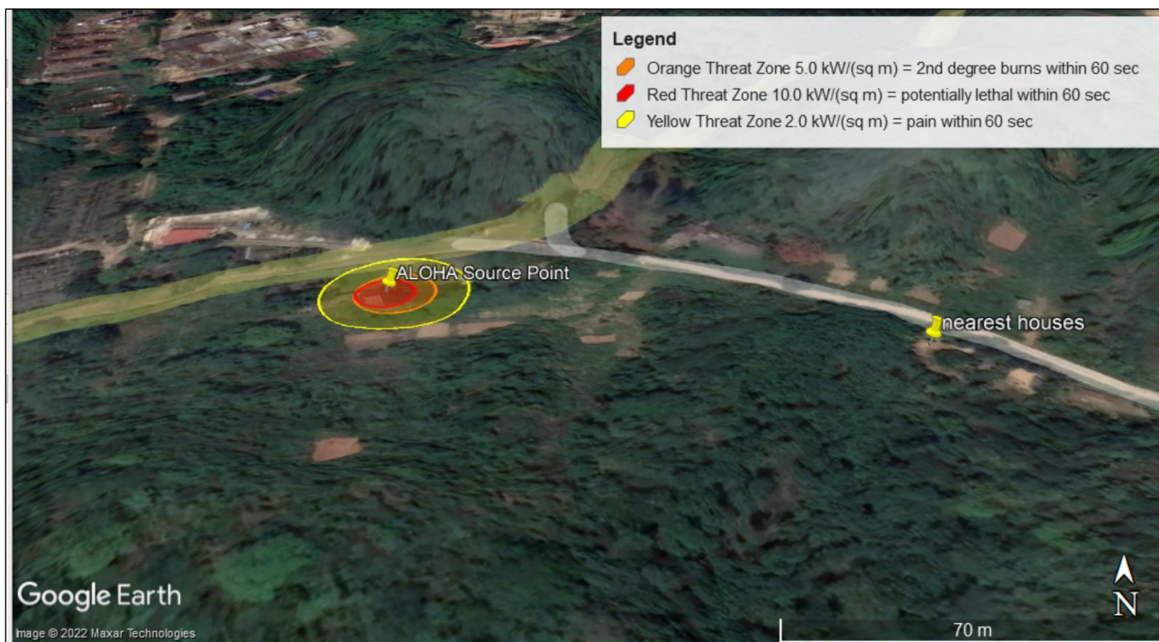
Figure 7-3: Location Map of Threat Zone of Thermal Heat Radiation of a Jet Fire from Gas Leak
